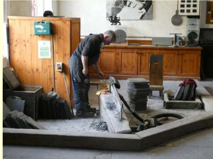
Hand splitting slate and cutting to size
